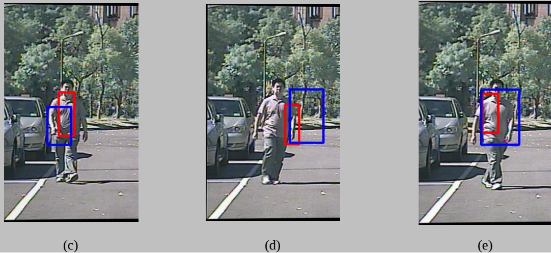
Figure 17. The tracking results of Kalman filter (blue) and particle filter (red) in different scenarios.
