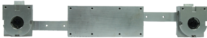
Figure 1. The flexible binocular stereo vision system with adjustable baseline length.
